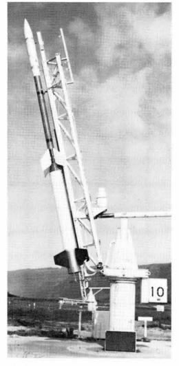
NITEHAWK 12 rocket vehicle, on its launcher at Barking Sands in Kauai, can carry a 220-lb. payload 100 miles above earth. The vehicle was developed at Sandia.
